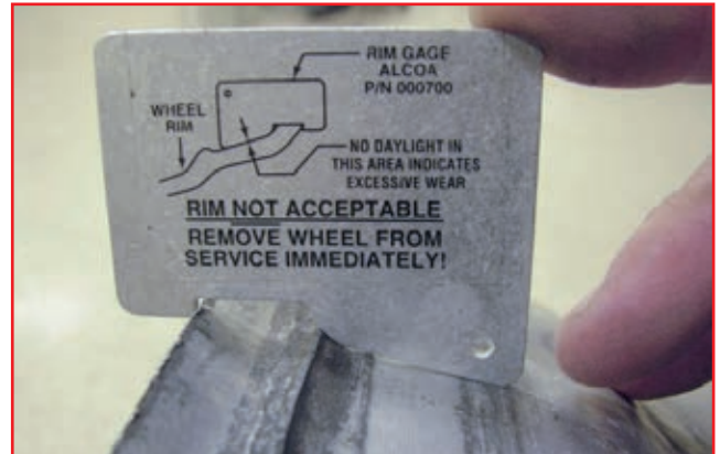
Picture 13-29 NOT SERVICEABLE
