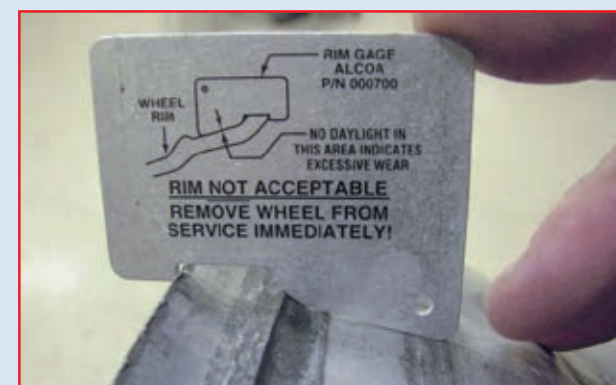
NOT acceptable rim flange wear
