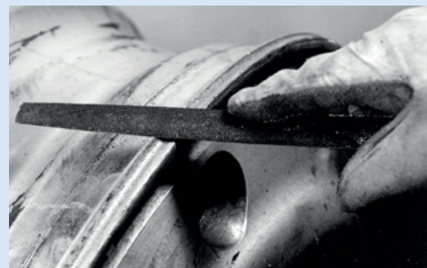
A file can be used very effectively to remove the sharp edge.
