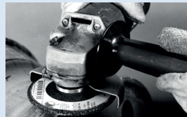
Use die grinder to remove metal. Do not gouge the wheel.
